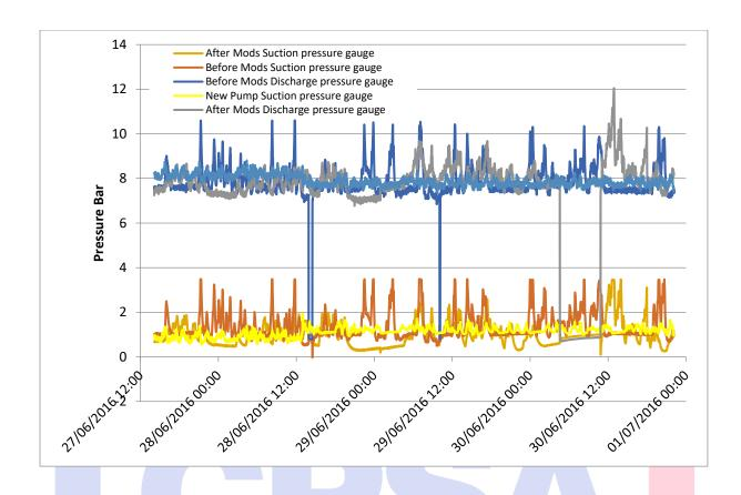
ERIKS established that the existing installed pumps were sized correctly for the insta<mark>llation</mark>, however site needed to ensure that the larger dynamometers received the correct flow and pressure by altering the control valve position as all the control valves were set to supply the correct flows and pressures for the smaller dynamometers.
